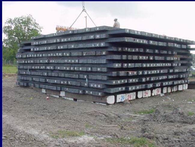
Cell A fully loaded with 1 million kilograms of steel (177 kN/m 2 )
